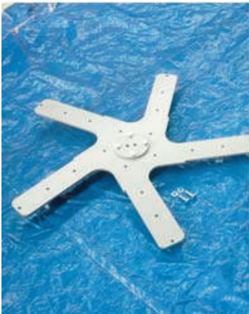
AFTER DISASSEMBLED BLADE SUPPORT, DISASSEMBLY HUB
